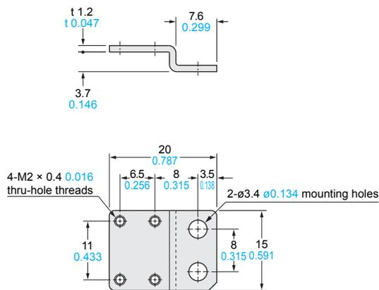
Material: Cold rolled carbon steel (SPCC)
