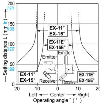
\*Optical properties of side sensing types (EX-“E”)
