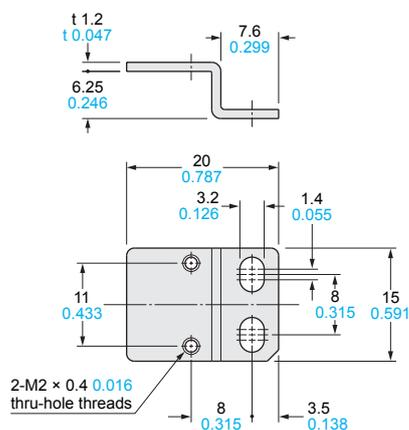
Material: Cold rolled carbon steel (SPCC)
