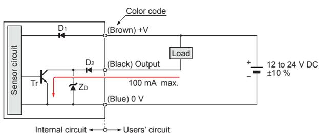
Symbols ... D1: Reverse supply polarity protection diode
